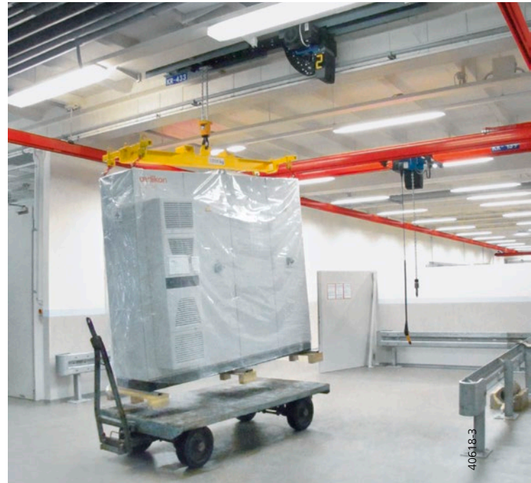
KLDC low-headroom travelling hoist with extended hook lead-off (for big bags)
